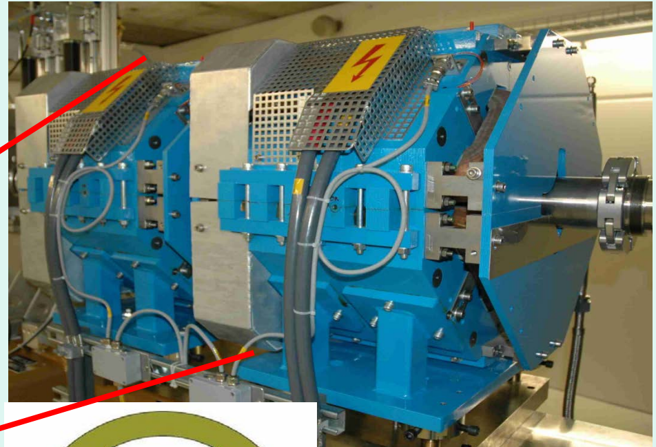
Quadrupole magnet: (de)focuses the beam
